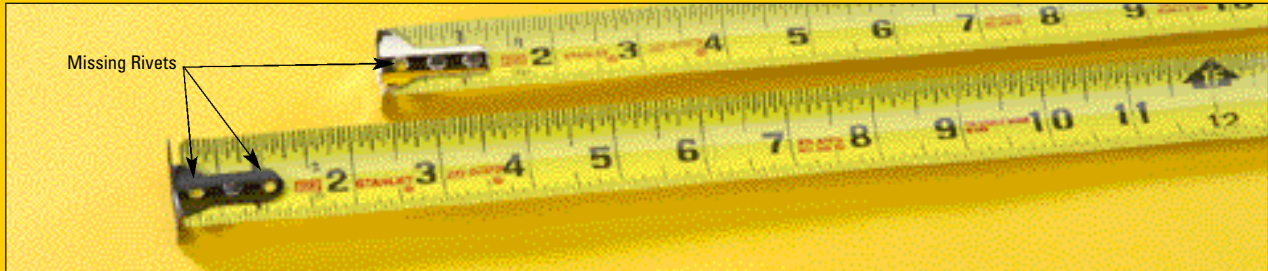
Missing Hook Rivets
